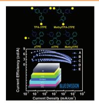
Five hole-dominated blue AIE molecules, constructed from TPA core and TPE derivatives peripheries, are successfully synthesized and serve as hole-transport layers and emitters for non-doped blue OLEDs with current efficiencies up to 8.03 cd A<sup>-1</sup>. By adopting construction approaches of changing linkage modes and increasing intramolecular torsion together, the conjugation lengths are effectively shortened for ensuring blue emission.
