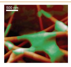
A simple, scalable, and relatively inexpensive method is described for preparing highly conducting AgNW/graphene hybrid transparent electrodes that use low-cost solution-processed pristine graphene. A combination of spray deposition and Langmuir-based techniques is used to produce ultrathin films with controlled nanowire and graphene densities. The results indicate that these graphene/ nanowire hybrid films may serve as a cheap replacement for existing technologies in electronic devices.
