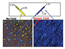
Kinetics of electric field induced alignment of anisotropic particles through the thickness of polymer film is studied using birefringence. Kinetics of alignment is used to determine the processing conditions to create continuous oriented films using roll-to-roll manufacturing process. The directional percolation of these particles enhances thickness properties creating functional films for membranes and flexible electronics.
