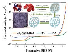
A simple, versatile and cheap synthetic route is developed for the preparation of Co<sub>3</sub>O<sub>4</sub> decorated blood powder derived foam-like heteroatom doped porous carbon (BDHC). The hybrid performs well as an advanced bifunctional non-precious metal electrocatalyst for oxygen reduction reaction (ORR) and oxygen evolution reaction (OER) in the alkaline medium.
