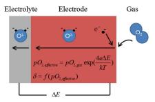
The non-stoichiometry of oxide thin films is systematically controlled by use of DC bias. The suitability of using bias across an electrochemical cell to conveniently and precisely control non-stoichiometry of oxide thin films, in an in situ fashion, and simultaneously monitor these changes by measurement of the chemical capacitance, is confirmed.
