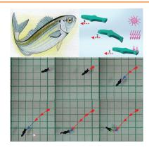
Soft and fast-response robotic platform constituted by PDMS/graphene-nanoplatelets composited layer (PDMS/GNPs) and pristine PDMS layer are proposed. The robotic platform can be driven by near infrared irradiation (nIR) due to the photothermal effect of graphene to mimic the fish swimming, which is hopeful in developing light-driven drug-delivery platform, but also the bio-robotic microgrippers applying in vivo and in vitro.
