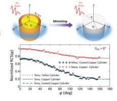
Quasi-three-dimensional and angle-tolerant electromagnetic illusion coatings are proposed, designed, and demonstrated using ultrathin single-layer functional metasurfaces with nonvanishing radial response. The quasi-two-dimensional metasurface coatings transform the electromagnetic perception of one object to mimic that of another which has been pre-selected by the designer. The illusion coating is realized using hundreds of composite electric and magnetic subwavelength unit cells.
